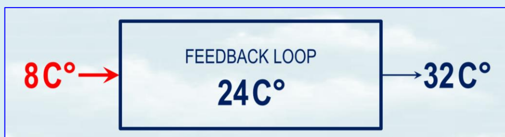
Fig. 7 Climate scientists imagine that the 8 C° direct warming by preindustrial noncondensing greenhouse gases drove a 24 C° feedback response. Their system-gain factor is thus 32 / 8 , or 4 : in other words, they multiply any direct manmade warming by about 4 to get final warming. Since the direct warming in response to doubled CO 2 in the air is approximately 1 C° , today's models predict about 4 C° eventual warming after accounting for feedback response.
